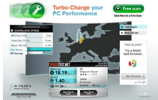
Speed test with PC connected to a modem, via a single JADE CMTS
